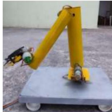
This robot is used for pick & place the object from one place another places. Concepts of automobile and robotics are combined in this project. It issued for assembly line, material handling etc. This robot does all those things it mainly reduces the manual work.
