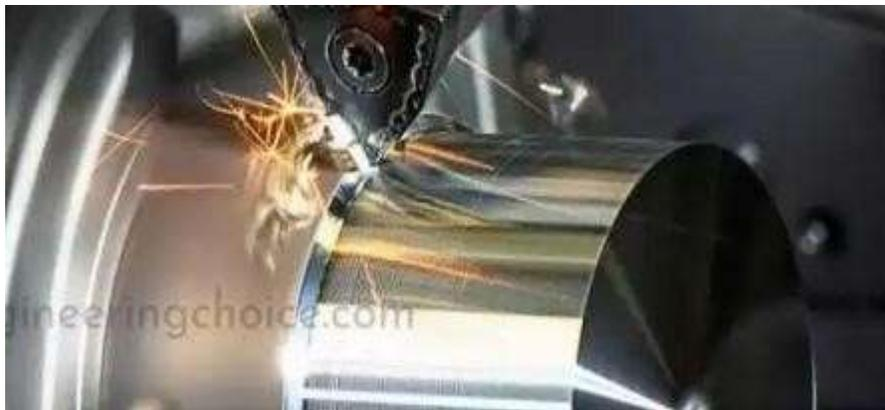
**Figure 1: Turning Process**
