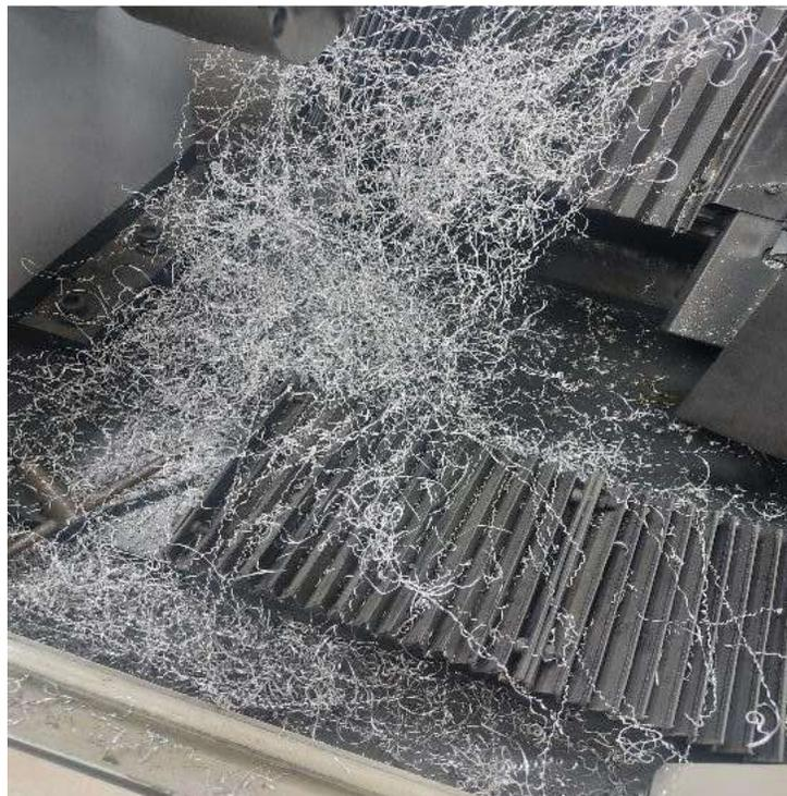
**Figure 11: Chip formed in turning process**
