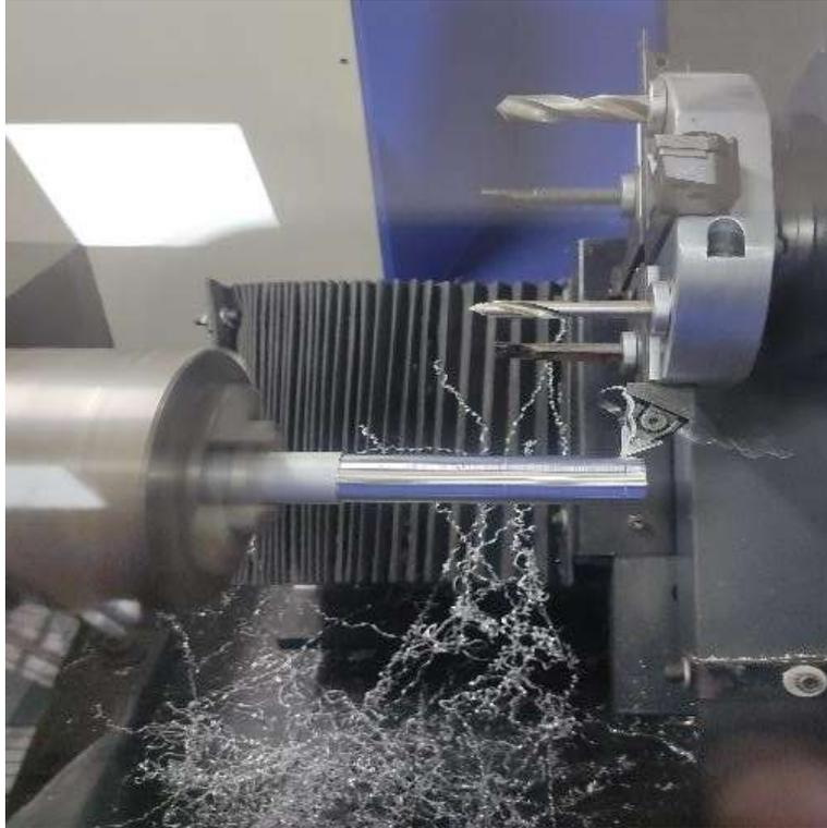
**Figure 10: Turning Process**
